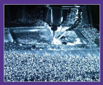
**E20** - A moderate-duty clear synthetic cutting and grinding coolant recommended for ferrous materials.
